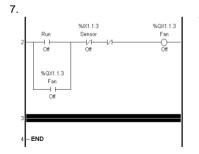
To insert a new rung below Rung 2, select Rung 2 and click on the  $\boxed{|+]}$  icon.
