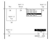
Drag the variable name "Fan" from Rung 2 and drop it onto the Normally-open contact in Rung 3.
